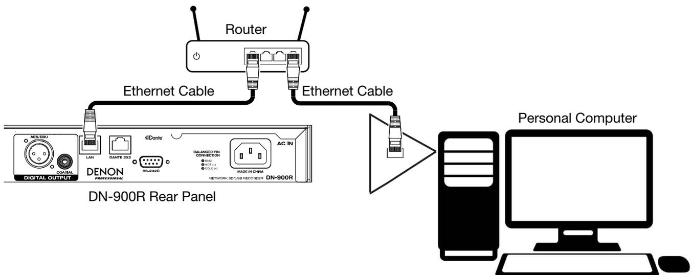
**Note:** Only one network user can be connected to DN-900R at a time. This means that two different computers cannot be used for serial communication with DN-900R at the same time, and you cannot use the LAN port for serial communication while DN-900R is already being controlled by the web browser remote.
