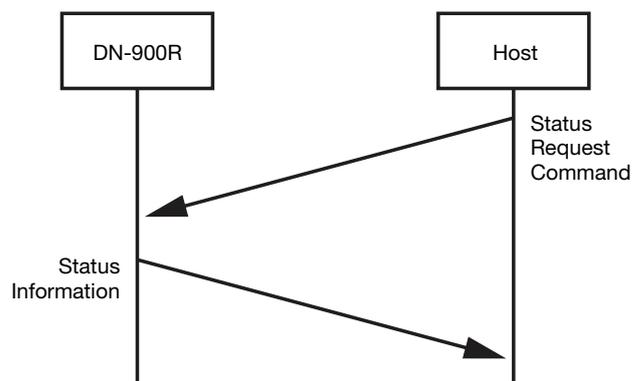
3. Status information automatically sent to the host when a change is made from DN-900R
